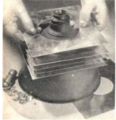
Above—Six square sheet-metal heat dissipators are attached to top of the lamphouse reflector.
