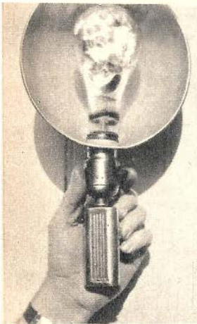
This flashgun was assembled from junk-box parts. The screw base from a flashlight bulb was soldered to the bottom of the socket and lead extended from short filament wire to socket terminals. To use, attach reflector and screw into a pocket flashlight. Right—A "dream effect" produced by means of a well-planned double exposed film.
