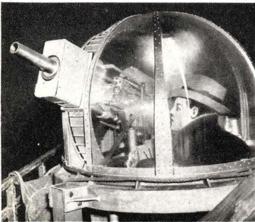
Flexibly mounted, enabling it to be aimed in any direction, this new airplane cannon fires a 37 mm TNT-filled shell.
