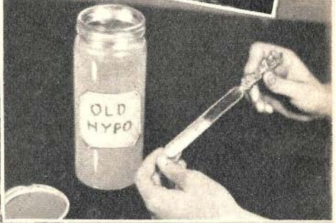
Cloudy hypo, no longer suitable for fixing purposes, can be used to give a silver plated appearance to articles of copper and brass. Clean metal well, immerse in hypo for 1 or 2 minutes, wash and finally polish with cloth.
