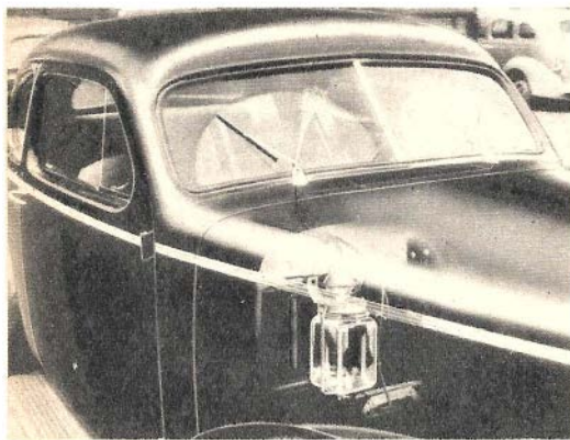
Mounted on the dash under engine hood, this cleaning unit ejects a fine spray of water on windshield at the mere pressure of a control button concealed on instrument panel.
