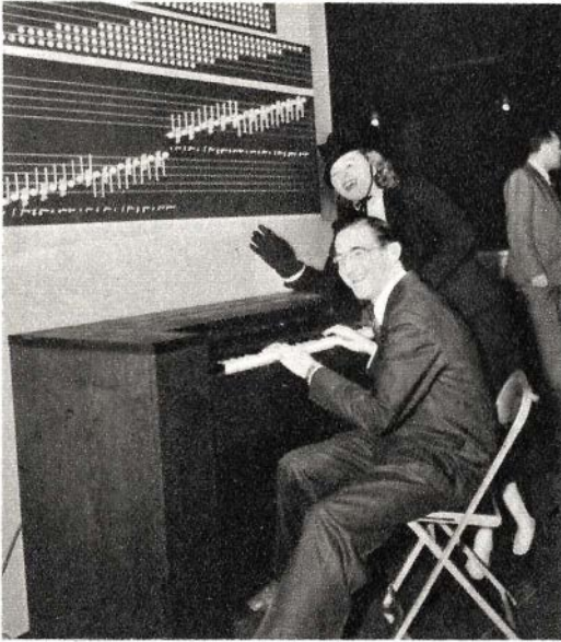
Silent practice is possible with this dummy piano, the keyboard causing "notes" to light up on the musical scale panel.
