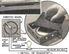
This sketch shows how to hook up a rheostat to control illumination provided by a photofood lamp. Right—Uncovered rheostat, showing simple parts.
