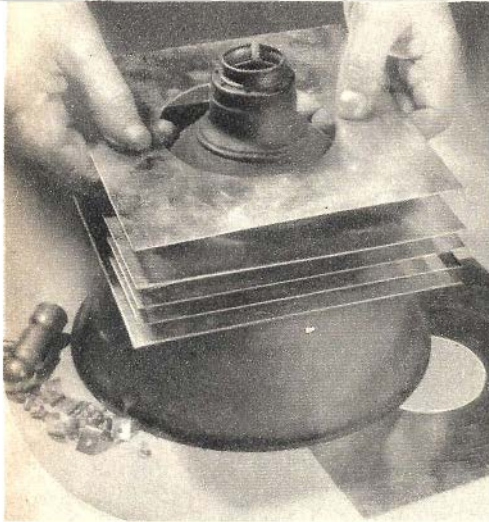
Above—Six square sheet-metal heat dissipators are riveted to top of the lamphouse reflector.
