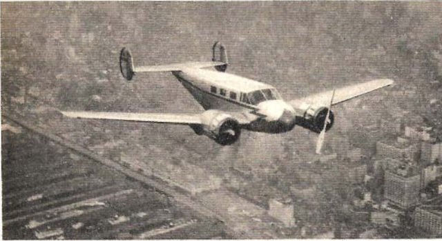
With one of its two 285-horsepower engines stopped, this Beechcraft transport plane flew 250 miles at 125 m.p.h.
