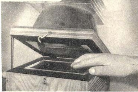
The negative may be placed or removed with ease, being merely laid on the mask as in contact printing (above). Left—Details of the lens focusing housing which telescopes over a felt-lined sheet metal tube. Right—Dimensions of the enlarger when designed especially for handling 9x12 cm negatives.
