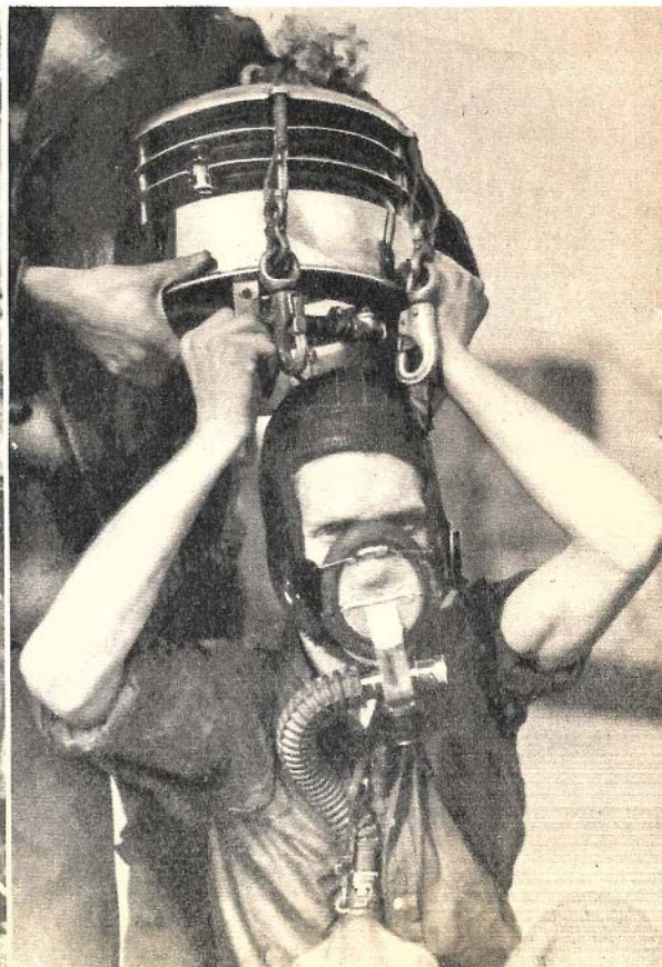
An ordinary football helmet protects Nohl's head against the diving helmet. The device over his nose separates carbon dioxide from the expired air.
