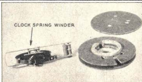
The fixture cord, which needs no special preparation, is doubled at the center, slipped through the rollers and inserted in the slotted center disc, as shown at left. By routing out the center of the middle disc and one hub, an alarm clock spring winder may be installed to provide an automatic rewind for the cord reel. Otherwise, reels can be wound by hand.
