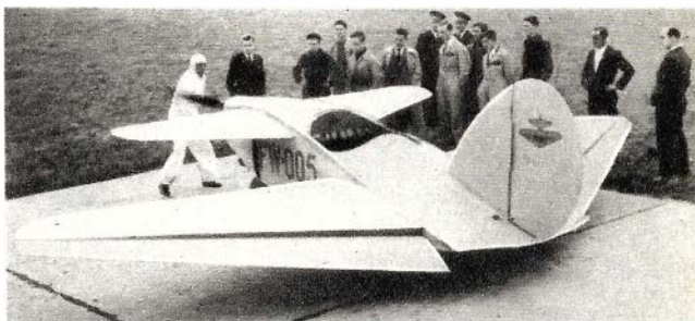
Presenting a novel appearance because of the peculiar arrangement of its wings, this French "flivverplane" is said to travel at 95 m.p.h. and has a cruising range of 350 miles.
