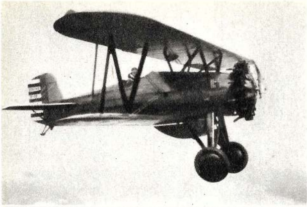
Produced in 1929, the P-12 single-seat, biplane pursuit plane (left) became standard equipment with the Army Air Corps. Later, as the F4B, this Boeing plane also became a standard U. S. Navy fighter.
