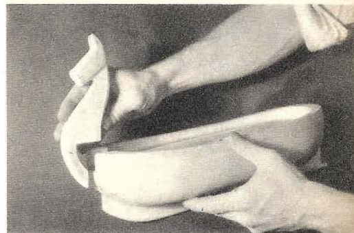
Photo 3.—Carve the figurehead and taper the bottom to blend in with the keel. Use 1-inch stock for this. Keel pieces are cut from \frac{1}{2} -inch stock, sanded smooth and glued in position.
