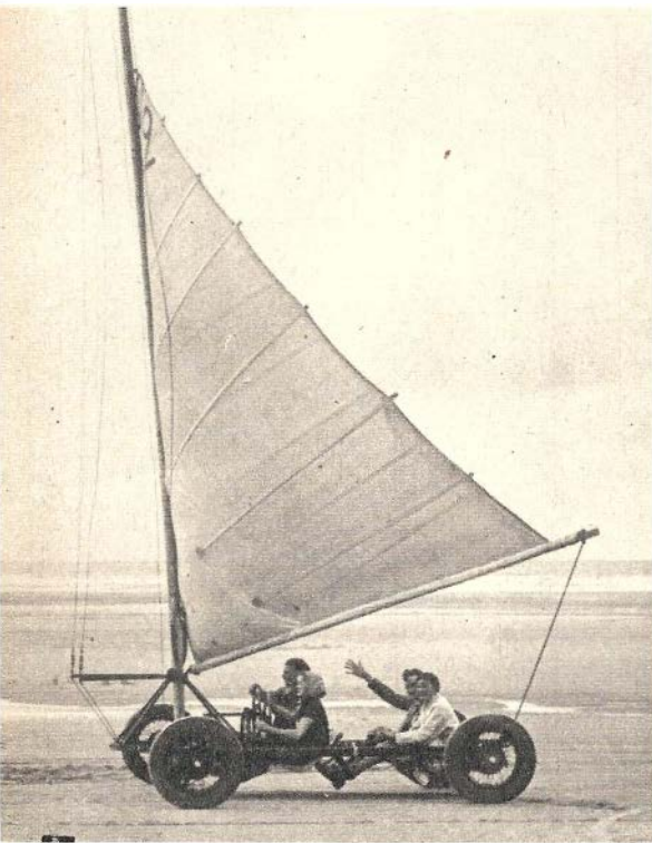
Plenty of thrills are provided for pleasure seekers who try their hand at navigating one of these sand yachts. Steering and sail control are achieved by means of dual hand wheels.
