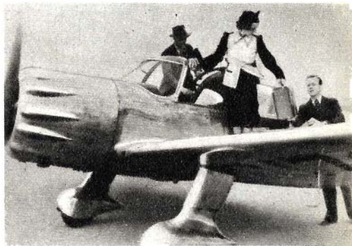
Constructed of glass, the sliding hatch of this sportplane not only enables the pilot and passenger to enter without stooping, but also provides excellent vision in flight.
