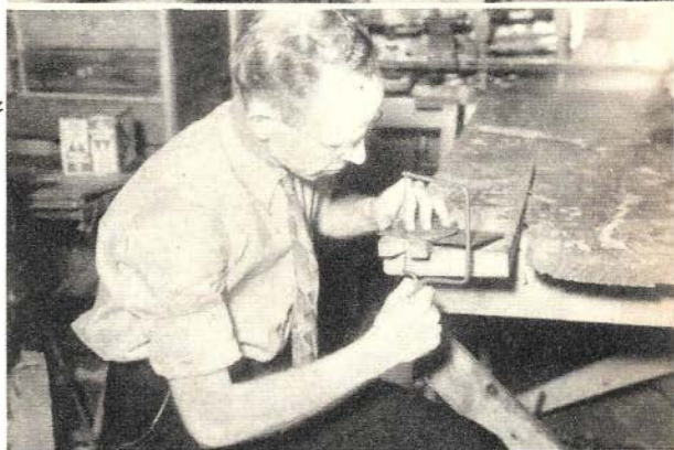
These pictures show the two methods by which old copper halftones may be cut into intricate shapes and designs. While a power jig saw will produce quicker and cleaner work, the hand saw is also practical.
