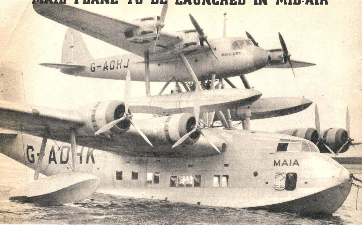
Carrying a load of 20,500 pounds, mail and fuel, the small seaplane component of this composite aircraft will be launched in mid-air from top wing of the larger plane, after which the small plane will carry its mail cargo from England to America.
