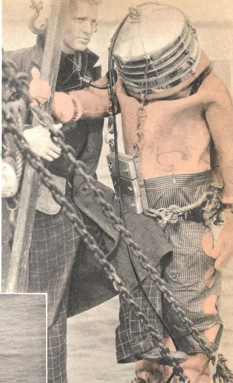
Not the Man from Mars, but Max Nohl as he appears in his flexible rubber suit with the oxygen and helium tanks strapped to his back. The valves at his left side permit convenient adjustment of the breathing components. He communicates with the surface man by means of telephone.
