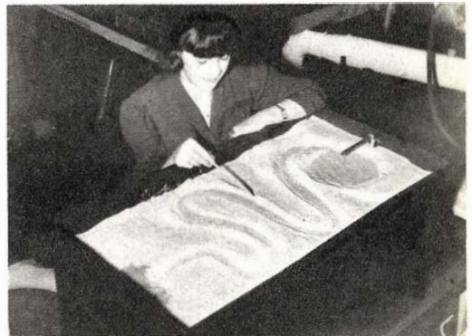
This test demonstration shows water passing through curves in chemically treated sand without becoming absorbed.
