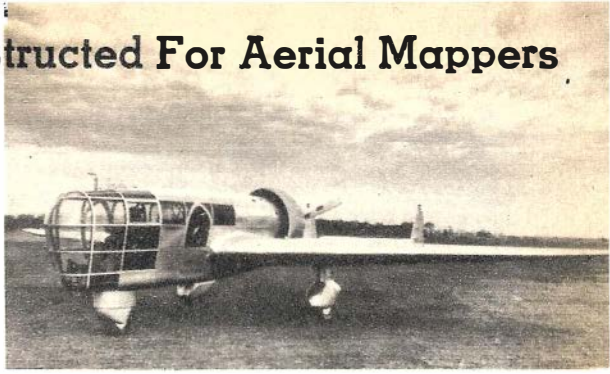
Featuring a glass nose, this airplane was designed for use by aerial mappers and photographers. The motor is mounted at the rear. Note the tricycle type landing gear arrangement.
