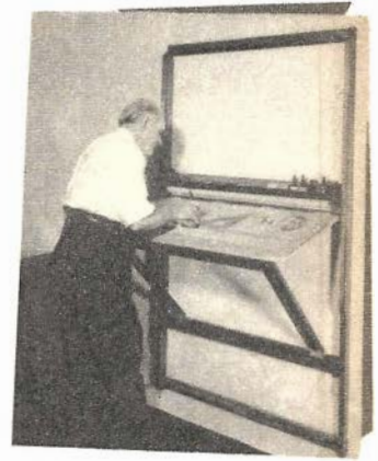
The tilting top of the drafting board is fully adjustable to any convenient angle. It may also be lowered to a vertical table-like position, 27 in. high.
