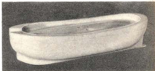
Photo 1.—The hull is built up from several pieces of pine stock, glued together, cut roughly to shape on a band saw. Final shaping is done with wood rasp and power disc sander.
