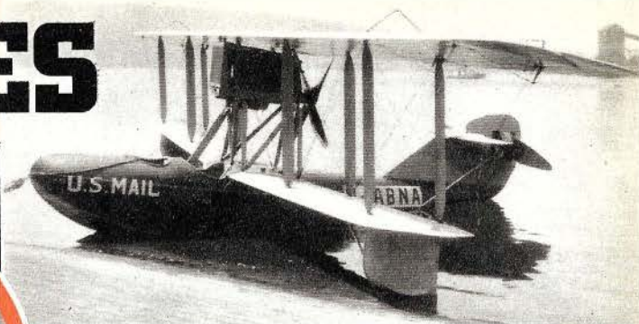
The Boeing B-1 flying boat (above), a pioneer mail carrier, was built in 1919. Still airworthy, it was retired from service after flying approximately 350,000 miles and wearing out six engines.
