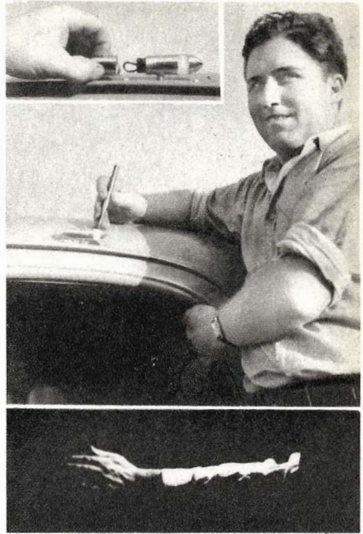
Housed in a metal shell (insert) mounted over driver's window (center), a compact electric light unit invented by Arthur Vaughn casts a beam on driver's signals at night (bottom).
