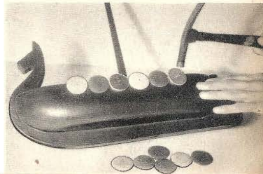
Photo 4.—Decorative shields, six on each side of hull, are cut from \frac{1}{4} -inch stock to a diameter of 1\frac{1}{2} inches. Sand one side so that they assume a convex shape, then nail in place.
